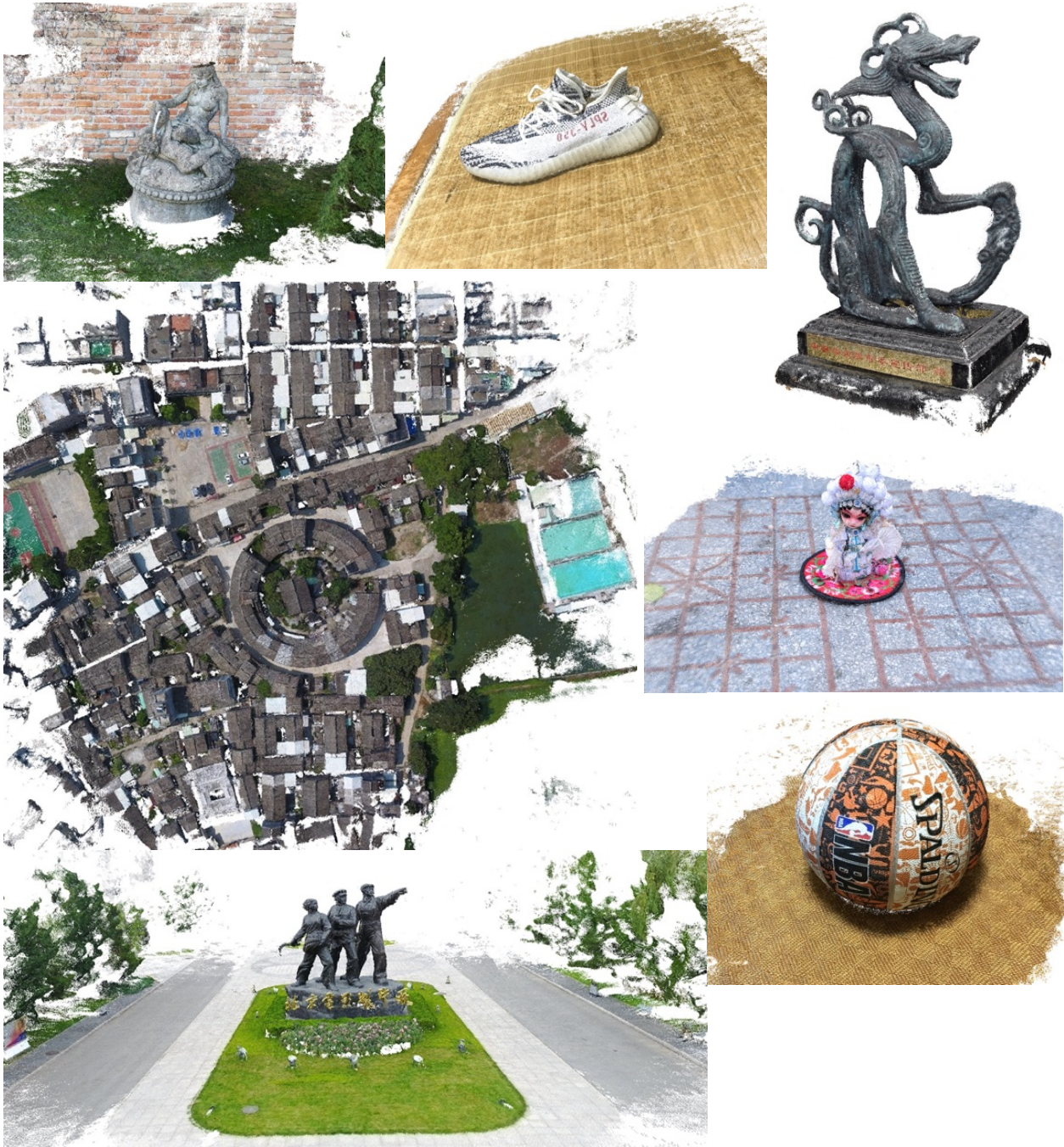
Figure 7. Point clouds reconstructed using GC-MVSNet for all scenes from BlendedMVS [18] evaluation set.
